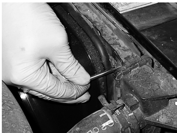
Install temp. probe near inlet hose...
